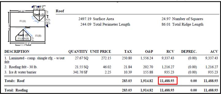
Figure 5: Showing the costs of a basic gable roof estimate, excluding ridge cap, starter, flashings and vents.
