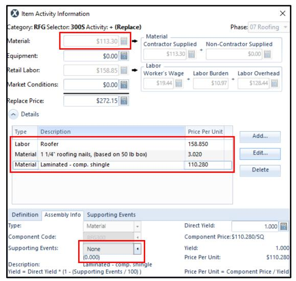
Figure 1: Showing material components of Xactimate line item 'RFG300S'.
